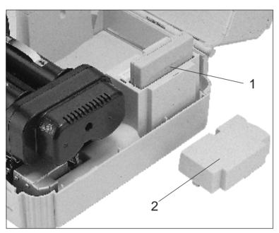
Fig. 10-1 Install Memory Module (Option)
